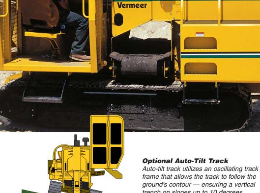
frame that allows the track to follow the ground's contour - ensuring a vertical trench on slopes up to 10 degrees.
