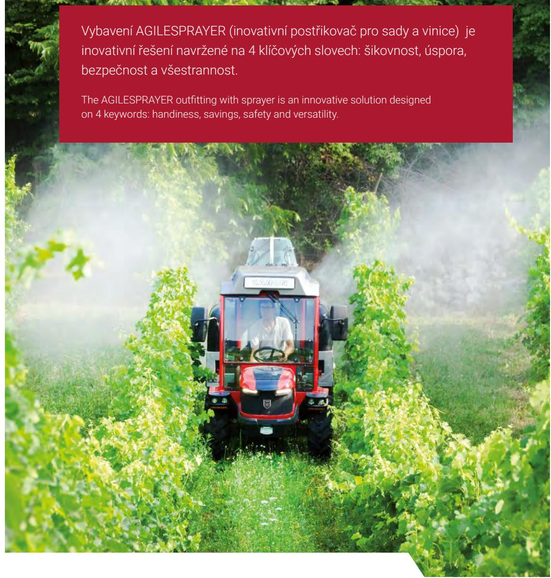
Thanks to agility, power and different equipment, AR/ST Series can be used in different contexts throughout the year. Models can be ordered with rear 3-point linkages, additional hydraulic distributors, Pto devices and drawbar hitch for different equipment such sprayers, forage self-loaders, tanks, manure spreaders, cranes, forest loaders.
